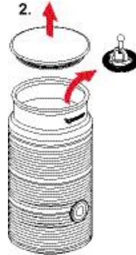
2) Remove lid and dismantle whisk.
