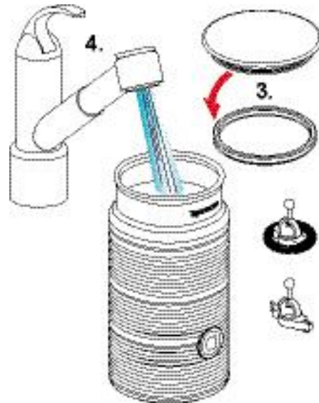
3) Remove seal from lid. 4) Rinse and clean milk frother together with whisk or mixer, lid and seal.
