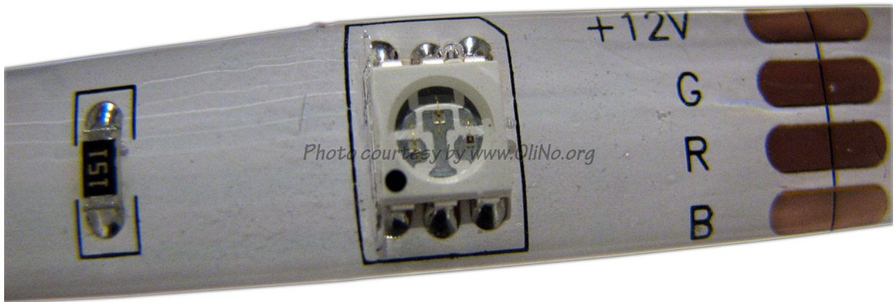
Detail photo of the RGB led on the flexible printed circuit board
