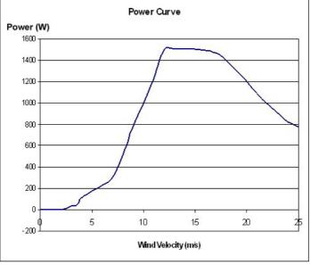
Figure 9 - Swift wind turbine power curve
