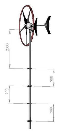
Figure 5 - Swift<sup>TM</sup> wind turbine assembly showing bracket spacings
