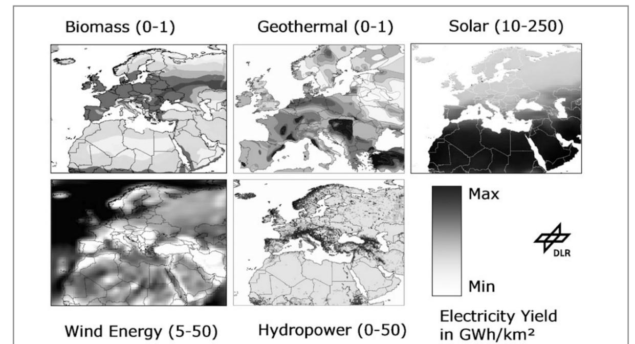
Figure 4: Renewable energy resource maps for EUMENA, showing the minimum and maximum annual electricity yield (as specified in brackets) that can be harvested by each technology from 1 km<sup>2</sup> of land area. Solar includes both photovoltaic and concentrating solar thermal power technologies. The overall potential and the different characteristics of each resource are given in Table 2 (MED-CSP 2005)
