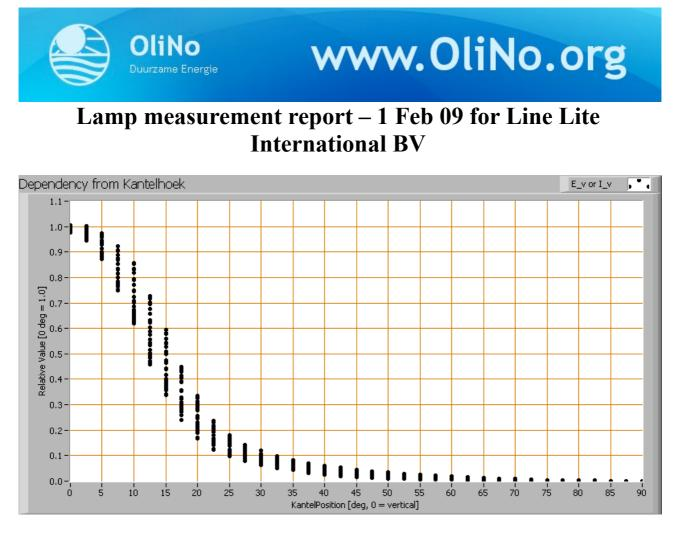
Intensity data of every measured turn angle at each inclination angle.
