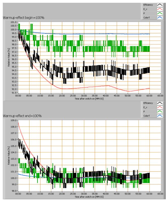
Effect of warming up on different light bulb parameters. At top the 100% level is put at begin, and at bottom at the end.
