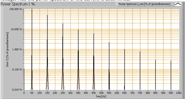
The powerspectrum of the current through the light bulb.
