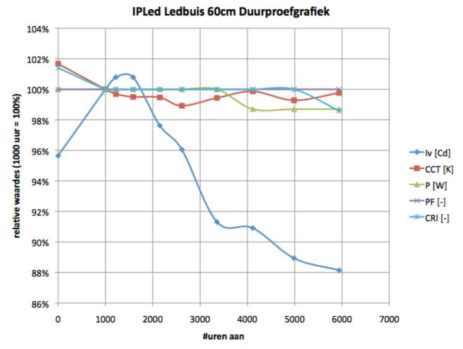
The variation of the lamp parameters during the endurance test.
