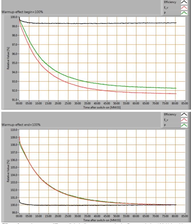
Effect of warming up on different light bulb parameters. In the first graph the 100 % level is put at begin, and in the last graph the 100 % level is put at the end.
